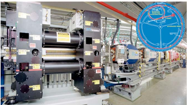
Storage ring: electromagnets
